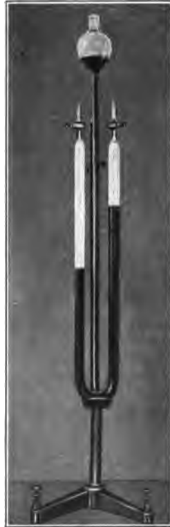
Apparatus for separating water by means of an electric current into the two elements, hydrogen and oxygen.
